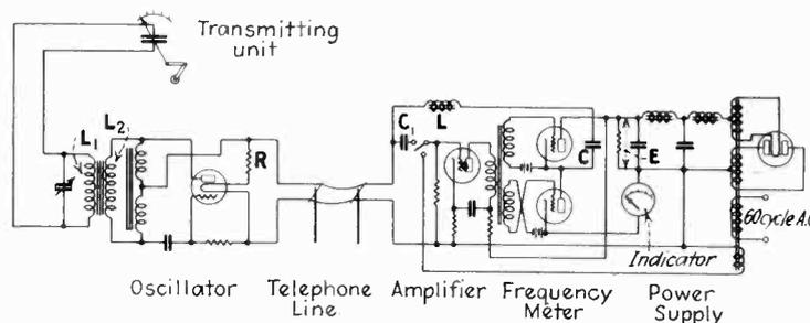
Circuit of transmitter and receiver
