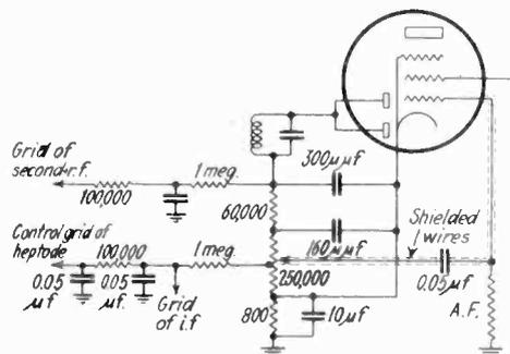
Anti-fading circuit employed in set criticized by French engineers
