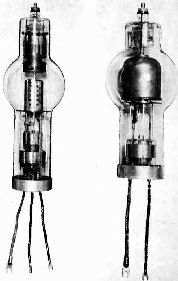
Types of Thyatron and Phanotron tubes used
