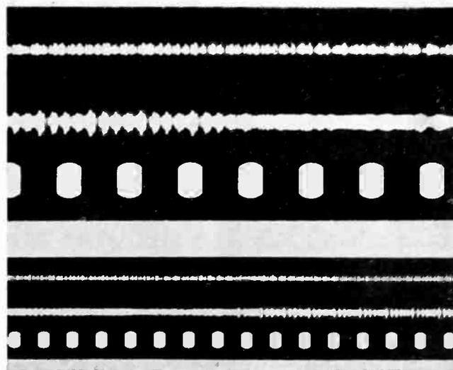
Enlarged samples of sound-tracks engraved by the mechanical recorder. The track at the bottom is actual size. Prints are made from these records in the usual manner
