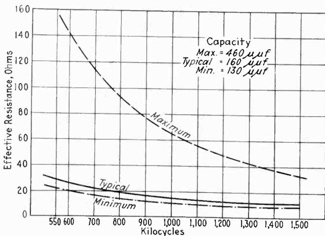
Fig. 3—Resistance characteristics of typical roof antennas
