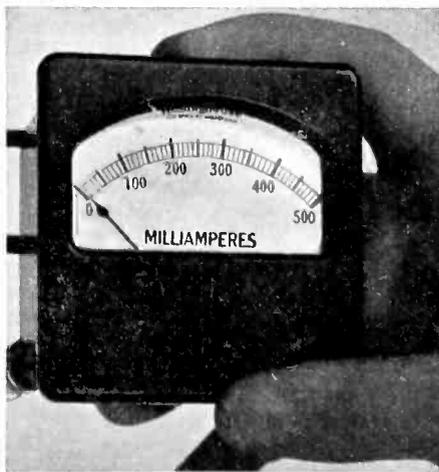
Refinements in the design of the movement of these meters are: soft iron pole tips welded to the permanent magnet in accurately aligned fixtures; improved springs; and an entirely new method of supporting the iron core in a die-cast bracket which uses jewel bearings. In the sensitive microammeters, strong cobalt steel magnets are used.—*Electronics*.
