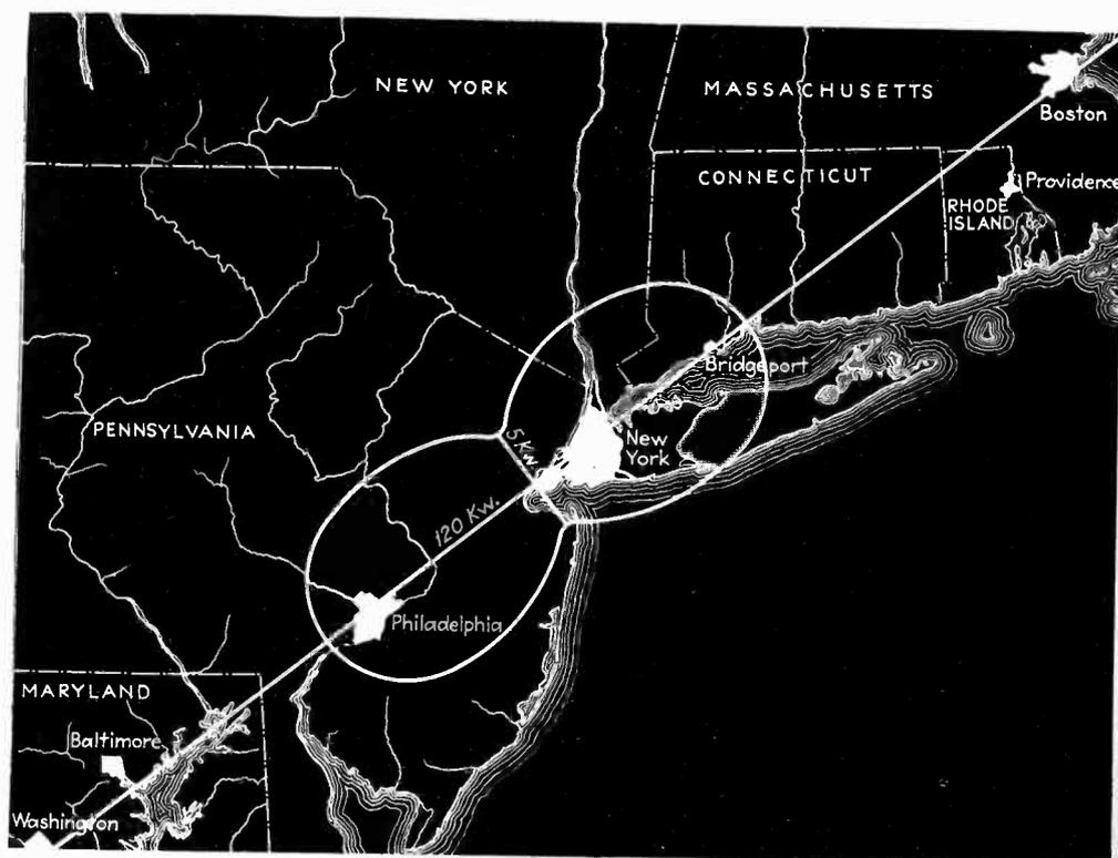
Relation of the new WOR signal to population. The hour-glass figure is the theoretical signal contour at one mile from the transmitting antenna, superimposed on the map of the service area. Note the amazingly large population centered on the axis of the 120 kw. signal
