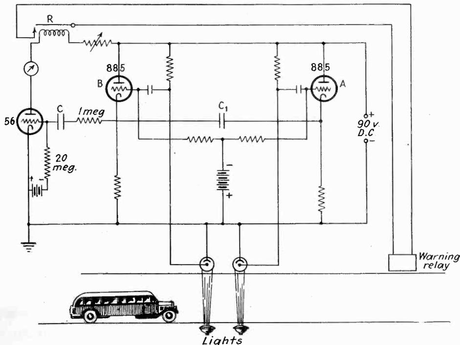
Circuit used in the photoelectric speed trap
