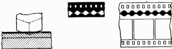
At left: The stylus cuts into a film having three layers. The bottom layer is the film itself, the middle layer a special material into which the stylus cuts, and the top layer a very thin opaque coating. Because of its wedge-shaped cutting edge the deeper the stylus cuts, the greater the width of the cut. Variable-width sound tracks of the kind shown to the right are produced when the stylus is controlled by a voice amplifier
