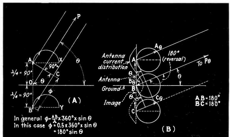
Fig. 4. (A) Doublet and image, expressed for the case of a doublet located one quarter wave above ground (cf. Fig. 5). (B) An antenna operated at its third harmonic, with current anti-nodes located at the ground and one half-wave length above it. (cf. Figs. 7 and 8.)
