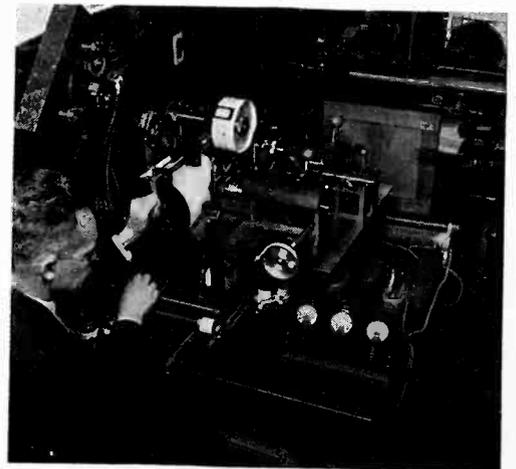
The photocell is used to measure spectrum photographs in this new comparator, invented by Prof. George R. Harrison
