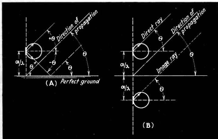
Fig. 3. In the diagram at the right, the effect of the ground reflections has been replaced by an "image doublet" located below the ground plane. The propagated waves in both cases are the same
