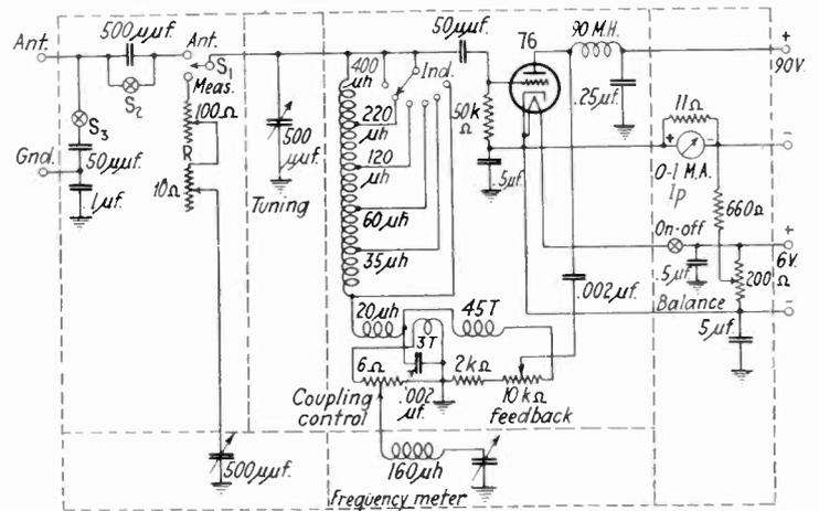
Fig. 2—Measuring set for antenna characteristics
