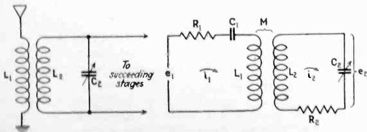
Fig. 1—Antenna and equivalent circuit
