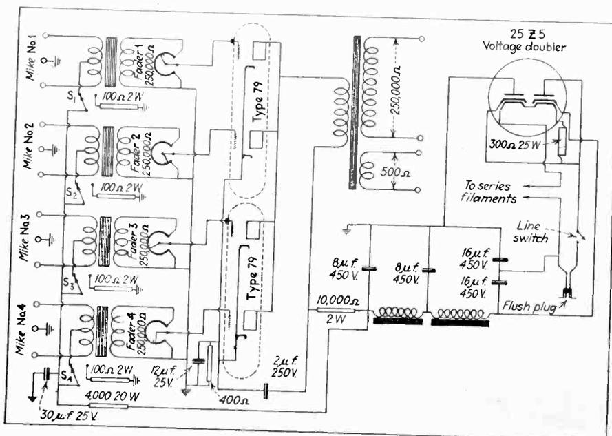
Electron-tube fader circuit
